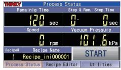
Displays real-time revolution speed and vacuum pressure
