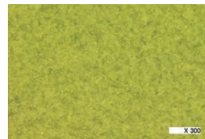
■ ARV-310LED Dispersion of orthosilicate fluorescent material (phosphor with about 15 μm particle diameter) and low viscosity silicone resin (3 Pa s) for LED
