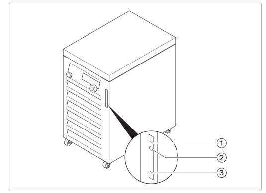
Fig. 5: Coolant fill level indicator
