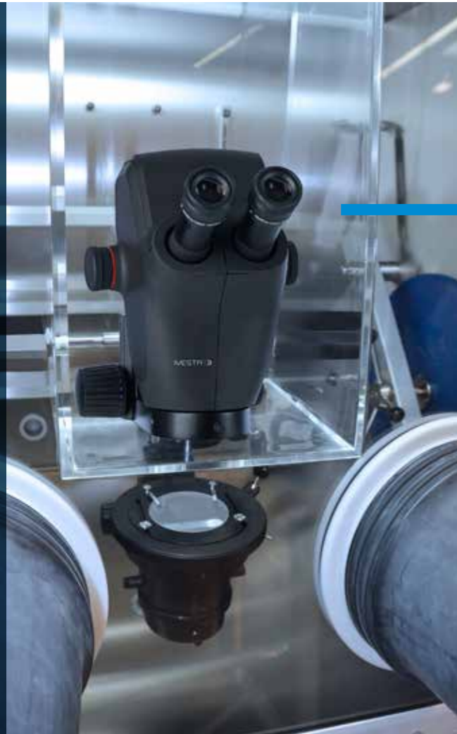
Complete Stereo microscope for the integration in MBRAUN glovebox windows.
